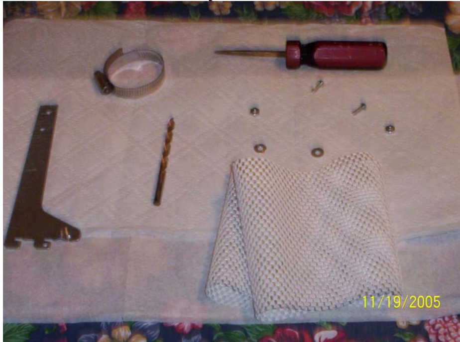
Figure 1.1: Adjustable Hose Clamp, Non Slip Grip Kitchen Mat, 3/16 Drill Bit, Single Track Shelf Bracket, Flathead Screwdriver, machine screws w/ nuts, and washers
