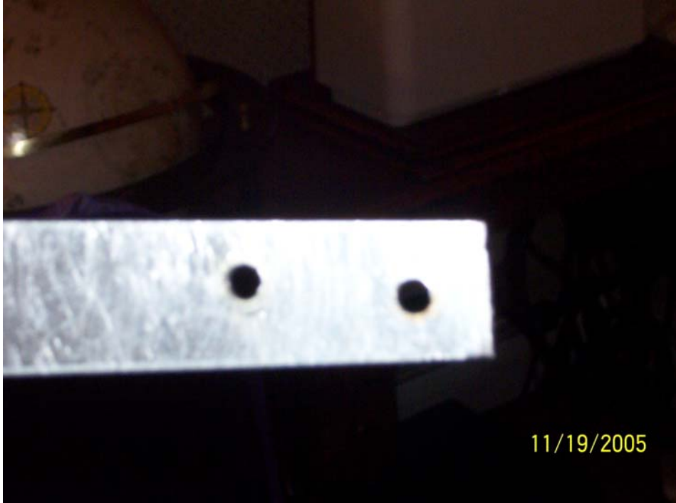
Figure 1.3: Drilled Holes in Single Track Shelf Bracket
