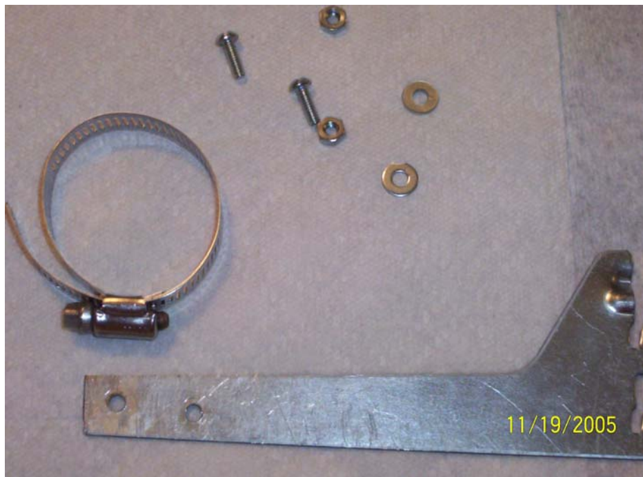
Figure 1.2: Adjustable Hose Clamp, Single Track Shelf Bracket, Machine Screws w/ nuts, and Washers
