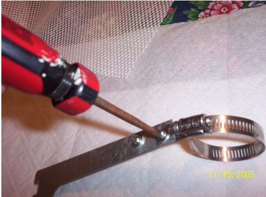
Figure 1.7: Screwing Machine Screws in Bracket and on Adjustable Hose Clamp
