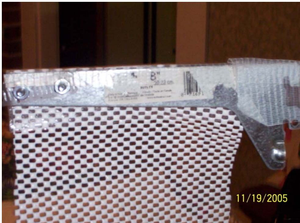
Figure 1.8: Attaching Mat With Clear Duct Tape
